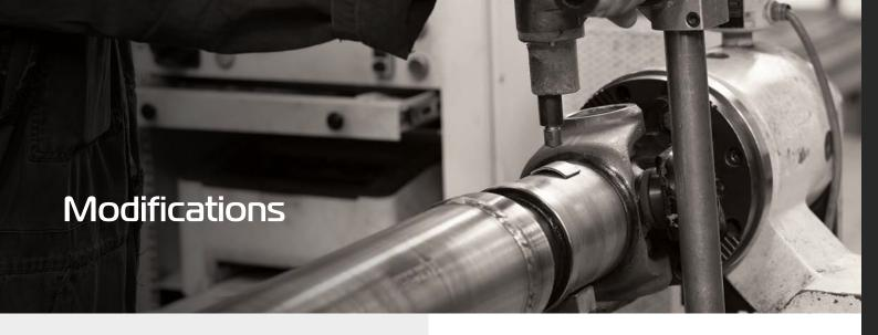
Due to the wide range of special purpose vehicles and equipment needed to meet the demands of many industries, we offer a modification service for all types of drivelines including shortening, lengthening of driveshafts and changing drive ends. This service is often used in applications such as chassis length adjustments and transmission or engine upgrades.
